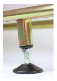
With Vauxhall deciding that you only needed roof mountings at the front and middle of your van, the aft-most crossbar uses a pair of adjustable rubber feet instead and has an extra M6 Nyloc nut and bolt at the end to prevent it from turning. Drop this into place but again, don't tighten everything fully yet.
